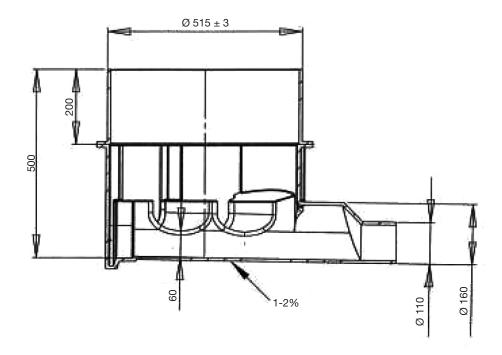
NOTE: As shown below, the side inlets are 60 mm higher than the main channel. Manhole chamber DN 500 mm height 500 mm
